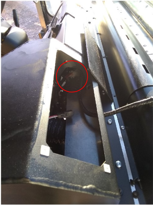
FIG 5 - CONTROL PANEL TO DUCT CONNECTION
