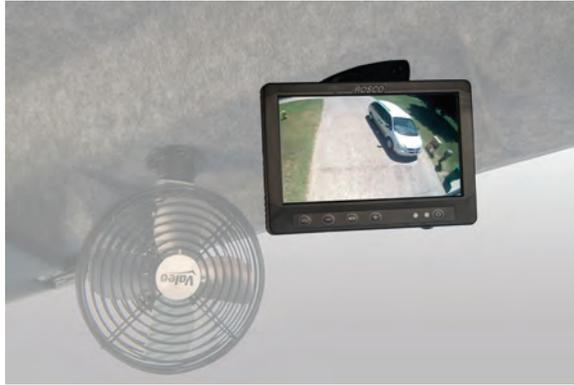
The rear view camera monitor is located above the windshield. The monitor provides a video image of the area behind your vehicle when the transmission is in reverse (R). A road side view camera also provides a video image of the area to the road side of your vehicle when the left turn signal is activated. See page 26 for the location of the rear view and road side cameras.
