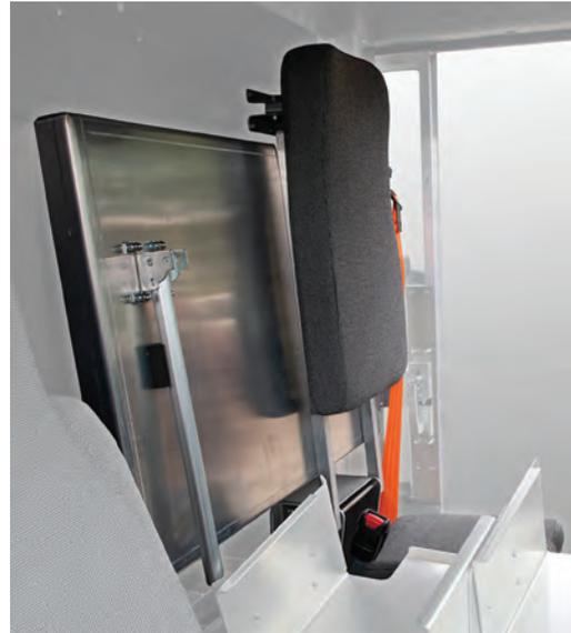
This vehicle may be equipped with a fold-down mail tray and passenger jump seat in the cab instead of a VTS. The support leg must be folded down when the mail tray is in use, and stowed when the tray is folded against the bulkhead wall. **NOTE:** The VTS and the fold-down mail tray cannot be used together. The VTS must be removed in order to use the fold-down mail tray.
