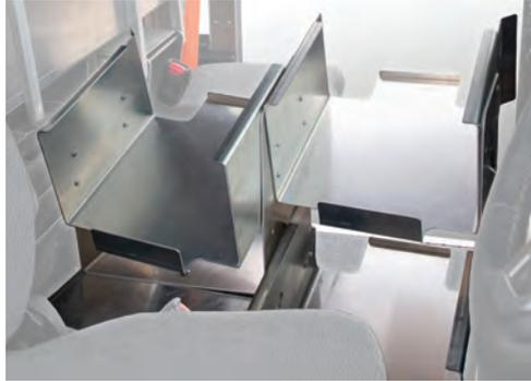
The vehicle tray system (VTS) is mounted to the cab floor and has space for three letterflatainers (LFTs), along with a secure collection bin (see below). Each tray is equipped to hold up to 40 pounds. The secure mail collection bin is loaded with a single LFT tray, which can be accessed from the roadside of the vehicle by unlocking with a vehicle key.
