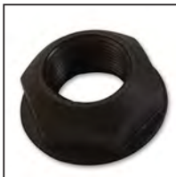
Retainer Nut P/N 47005901 Tighten to 20 ft/LBS.
