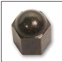
Acorn Nut P/N 81600189 Tighten to 20 ft/LBS.
